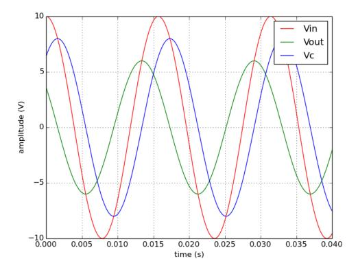
Here we can see that the output voltage leads the input and the capacitor voltage lags the input. The Python code can also be used to verify that, for all t, the sum of the resistor and capacitor voltages equals the input voltage.
