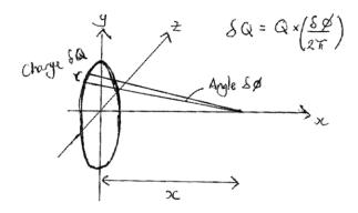
The diagram shows an element of charge,  $\delta Q$ , that subtends an angle  $\delta \phi$  as shown. As the charge on the hoop is uniformly distributed its value is thus  $\delta Q = Q \frac{\delta \phi}{2\pi}$ .
