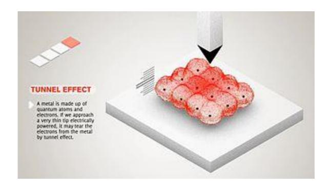
It is the basis of the Scanning Tunnelling Microscope (STM). In this device as an atom scale tip is scanned across a surface the tunnelling current is modulated by the atomic scale features, thus mapping the surface with atomic resolution. (Invention awarded the Nobel prize in 1986)
