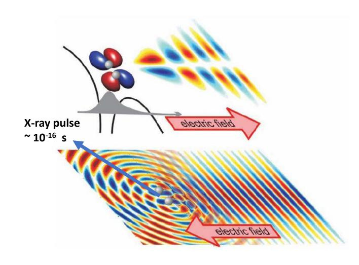
The duration of the tunnel current is typically  $\sim 10^{-16}$  s and can give rise to sub-fs pulses of X-rays perfectly synchronized to the laser field
