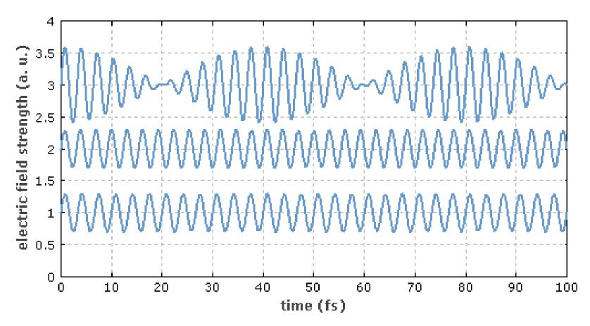
A beat note at  $(\omega_1 - \omega_2)$  is synthesized from two continuous monochromatic fields of frequency  $\omega_1$  and  $\omega_2$
