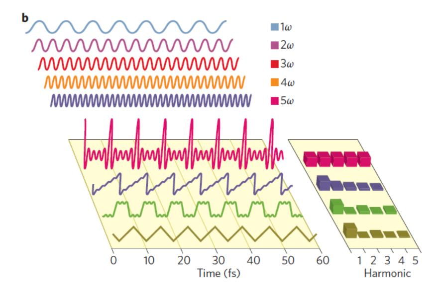
A periodic waveform with high temporal resolution features can be synthesized from multiple octave spanning components of a superposition of fields (e.g. here from integer multiples of the fundamental frequency  $\omega$ )
