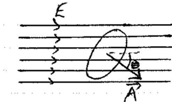
Figure 3.1 A uniform electric field intersecting an area at an angle to it
