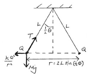
Vertically the weight of the sphere is exactly balanced by the vertical component of the tension in the string i.e.  $mg = T\cos\frac{\theta}{2}$  so the value for the tension in the string is  $T = \frac{mg}{\cos\frac{\theta}{2}}$ . This makes sense as when the angle is zero the tension is equal to the weight and as the angle approaches  $180^{\circ}$  it becomes progressively difficult for the vertical component to match the weight hence it tends to infinity.
