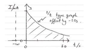
As current is defined by  $I = \frac{dq}{dt}$  the charge that has passed is given by the area under the curve.
