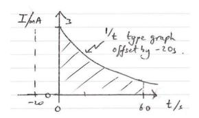
As current is defined by  $I = \frac{dq}{dt}$  the charge that has passed is given by the area under the curve.
