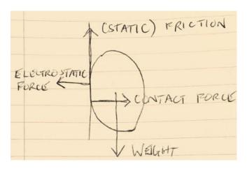
Clearly the friction must equal the weight and the electrostatic force must equal the contact for for linear equilibrium but notice the relative positions of the forces needs to be in the sense noted for rotational equilibrium as well.
