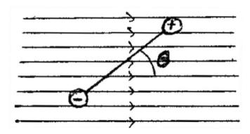
Using the rotational form of Newton's second law, i.e.  $\Gamma = I \frac{d\omega}{dt}$  and the dynamics of the situation showing the magnitude of the torque on the dipole to be  $qEd\sin\theta$  and always acting to restore the dipole to equilibrium, it can be written  $I \frac{d^2\theta}{dt^2} = -qEd\sin\theta$ .
