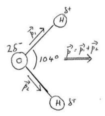
In this representation the oxygen atom is thought of as two overlapping point charges, each of value  $-\delta$ , and each hydrogen atom is thought of as a point charge of value  $+\delta$ .
