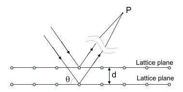
i) Using the figure above, show that the path difference between waves scattered from atoms in adjacent planes is  $2d \sin \theta$ . Note that it is customary to measure  $\theta$  from the lattice plane and *not* relative to the normal to the surface.
