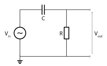
Hint: It can be useful to represent the three voltages (input, capacitor and resistor) as functions of time and then plot these using Python. You can then check your answers against a simulation of the circuit in LTSpice. This is **not** required to be given as part of your answer, however.
