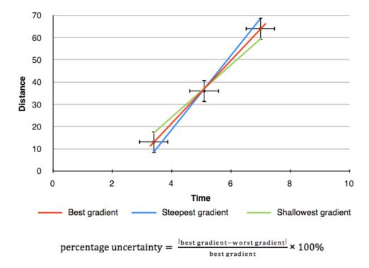
To determine the uncertainty in the y – intercept we do the same thing as when calculating the uncertainty in gradient. This time however, we check the lowest, highest and best value for the intercept by drawing the different possible intercepts from the different gradients.
