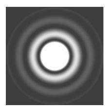
Students should be able to link the picture above with the graph below. The vertical axis is intensity or brightness, and the horizontal axis is angle,  $\theta$ , or  $\sin \theta$ . For small angles these two are approximately equal, if  $\theta$  is in radians.
