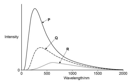
The graph shows that the hottest object (P) has a peak at the shortest wavelength. In fact, the relationship between the wavelength of the peak,  $\lambda_{max}$ , and the temperature, T, is called Wien's displacement law:
