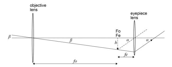
It should be clear from this diagram that the angular magnification is  $\frac{\alpha}{\beta}$ , and that the image is inverted.
