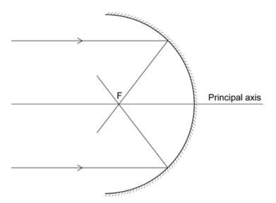
Unfortunately, circular (or spherical) mirrors are not so simple. Off-axial rays are brought to a focus closer to the mirror. This means that the focal point is different for different rays of light. This results in a blurred image and is called spherical aberration. This ray diagram is obtained fairly easily by following the reflection law, having drawn a circular mirror on a piece of paper.
