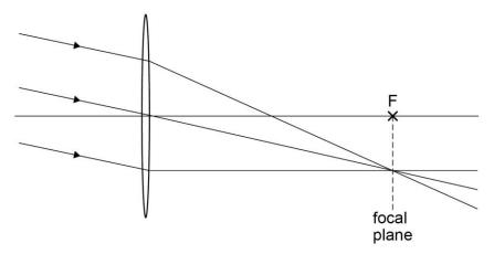
Notice that, with this thin lens, the rays are only shown bending in the middle of the lens, and that the central ray passes straight through without bending.
