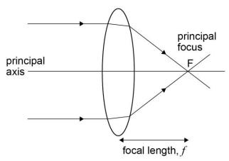
The refraction of the light passing through the lens is shown in this diagram. When drawing ray diagrams, the situation is simplified by assuming that the lens is very thin so that the ray is only shown bending once, in the middle of the lens.
