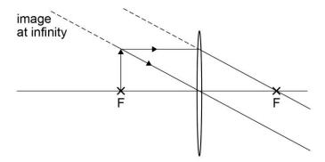
In this situation, the rays leave the lens parallel. The image can only be seen by looking through the lens – it is a virtual image at infinity.
