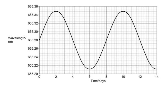
The peak in the graph (at 656.35 nm) occurs when the star is receding from our point of view, at its maximum velocity, ie the two stars are next to each other. The eclipses occur when the star is moving at right angles to our line of sight and the wavelength is 656.28 nm.
