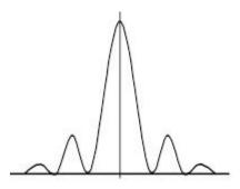
For a single slit, minima in the pattern are at angles given by
