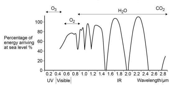
This graph shows the effect that water vapour, carbon dioxide, oxygen and ozone have on the IR, visible and U-V spectrum as the radiation passes through the atmosphere. This explains why telescopes detecting these parts of the em spectrum are placed on balloons, in orbit, at the top of high mountains, or in very dry areas (such as the Atacama Desert).
