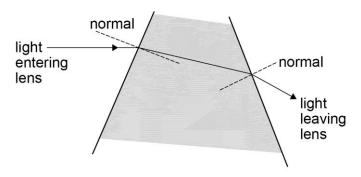
A convex lens is designed to have the correct curvature needed to bring parallel light to a point focus. This diagram shows light entering a lens parallel to an axis of symmetry called the principal axis. Such rays of light are called axial rays. The point on the axis where the rays cross is called the principal focus, F.
