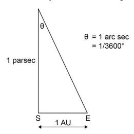
The parsec is an important unit because of the way distances to nearby stars can be determined – trigonometrical parallax. This involves measuring how the apparent position of a star, against the much more distant background stars, changes as the Earth goes around the Sun.
