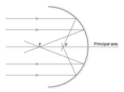
The problem of spherical aberration is overcome using a parabolic mirror (the more mathematical students may recognise a parabola as an ellipse with one focus at infinity).
