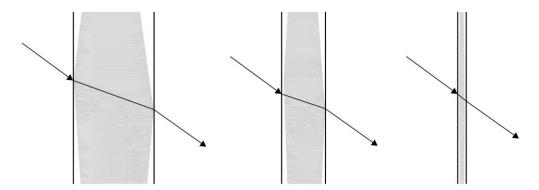
This diagram shows that, as the lens is made thinner, the path of the ray through the centre of the lens is deviated less. This is useful in ray diagrams because the path of this ray can be drawn as a straight line when the lens is thin.
