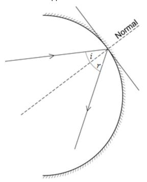
This leads to the idea that a concave mirror will bring parallel light to a point focus. The focal point, F, is taken to be at half the distance to the centre of curvature.
