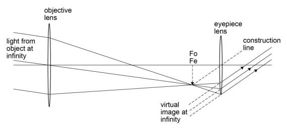
The telescope is in normal adjustment because the image is formed at infinity, ie the light rays leave the telescope parallel. This means that the focal points of the two lenses coincide, making the distance between them equal to the sum of the focal lengths.
