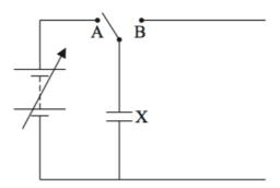
When the switch is connected to terminal A the capacitor X is connected to the variable power supply.
